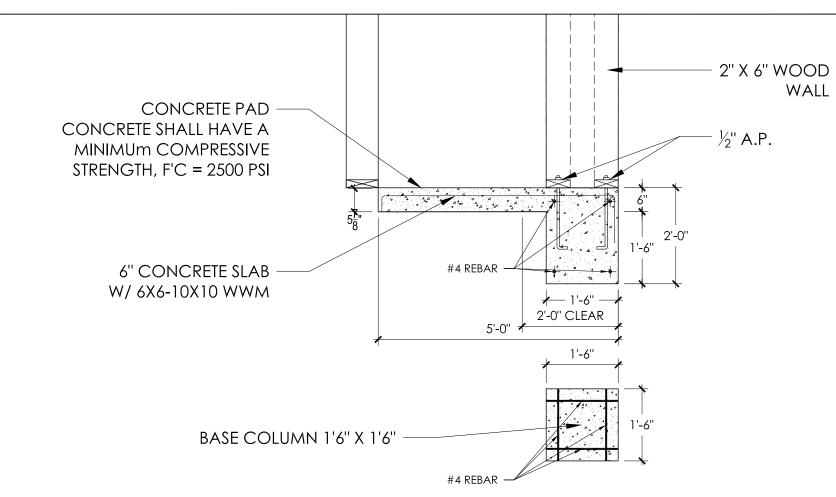
DETAIL COLUMN FOOTING AND SLAB
