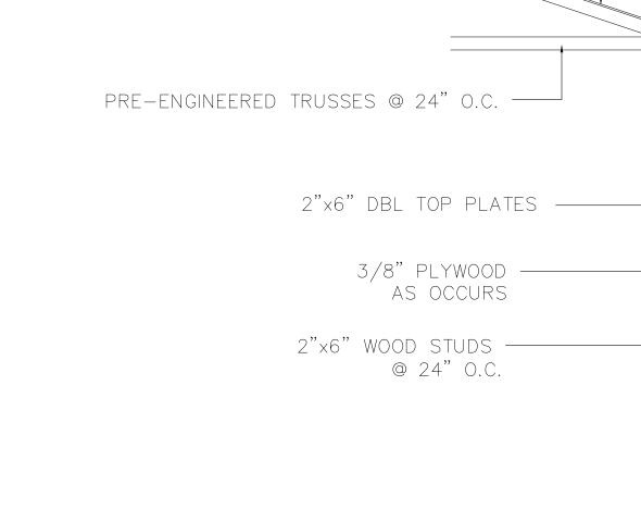
2"x6" WOOD STUDS -@ 24" O.C. 3/8" PLYWOOD -AS OCCURS 2"x6" SOLE PLATE —
